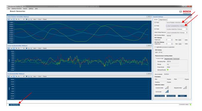
You should now see quaternion data with 200Hz Output data rate, Linear acceleration with 100Hz Output data rate, both at 100Hz Refresh rate.
