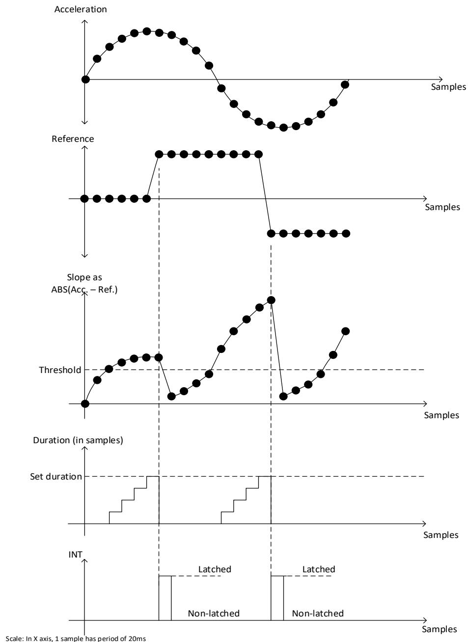
Figure 1: Any-motion detection
