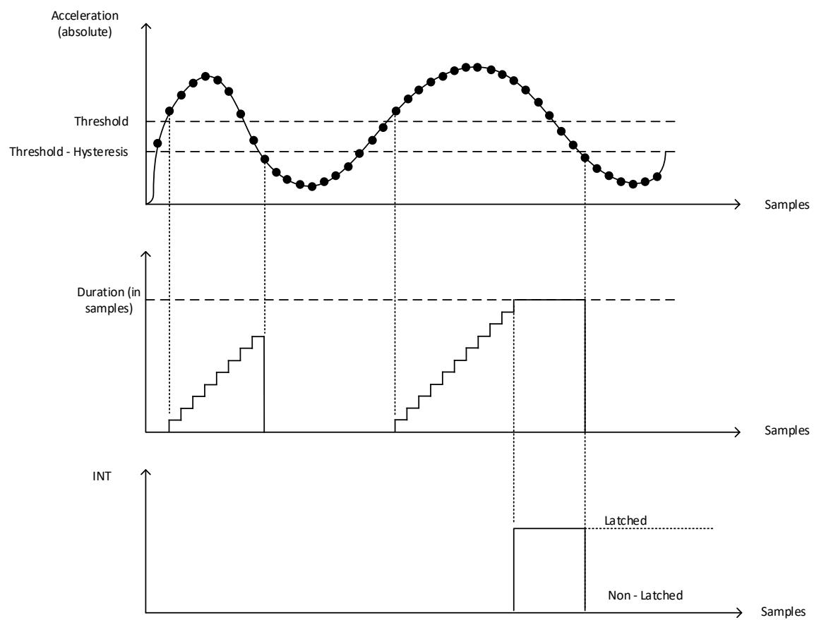
Figure 7: High G detection
