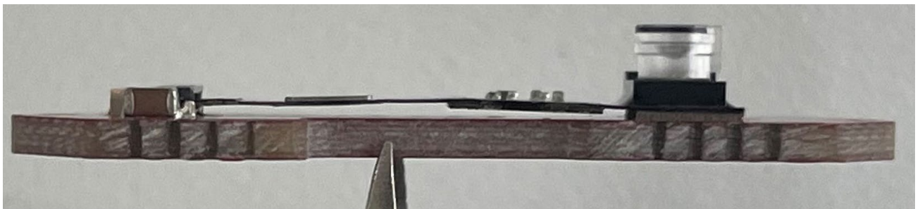
Figure 20: Depiction of proper thermal connection
