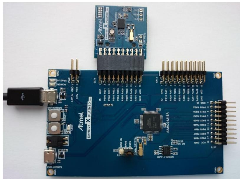
**Figure 1 - Main and Extension board connections**
