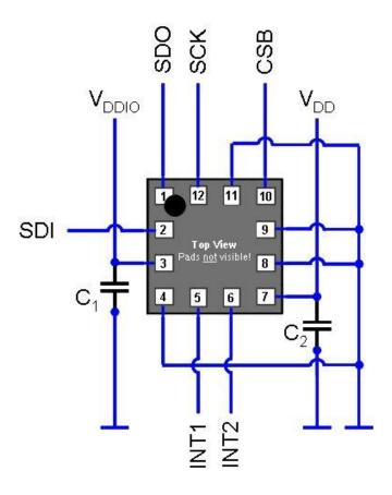
Figure 24: 4-wire SPI connection
