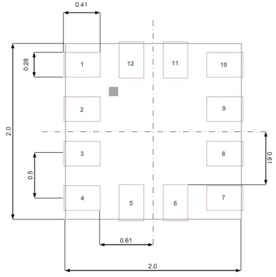
Figure 29: Landing patterns; dimensions are in mm
