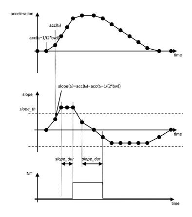
Figure 7: Principle of any-motion detection
