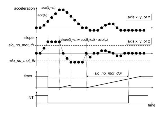
Figure 11: Timing of No-motion interrupt
