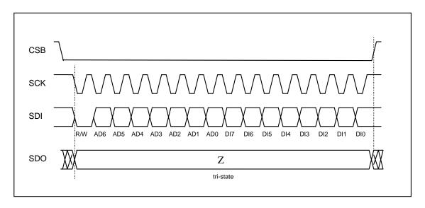
Figure 14: 4-wire basic SPI write sequence (mode '11')
