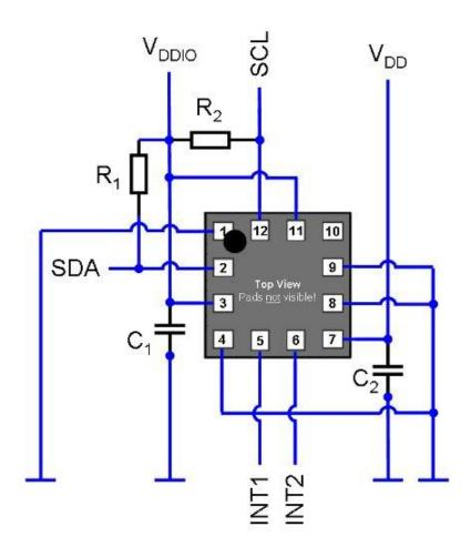
Figure 26: I<sup>2</sup>C connection
