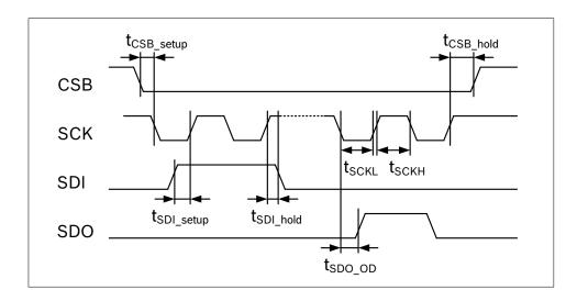
Figure 13: SPI timing diagram
