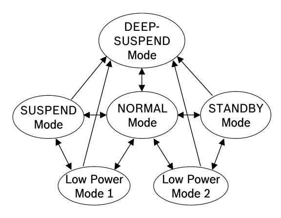
Figure 2: Power mode transition diagram
