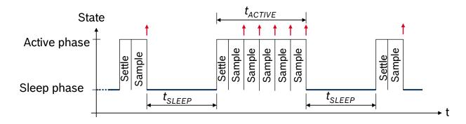
Figure 3: Timing Diagram for low-power mode 1/2, EDT
