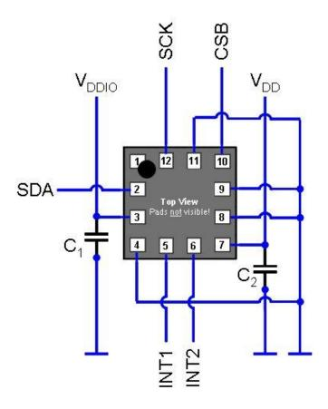
Figure 25: 3-wire SPI connection
