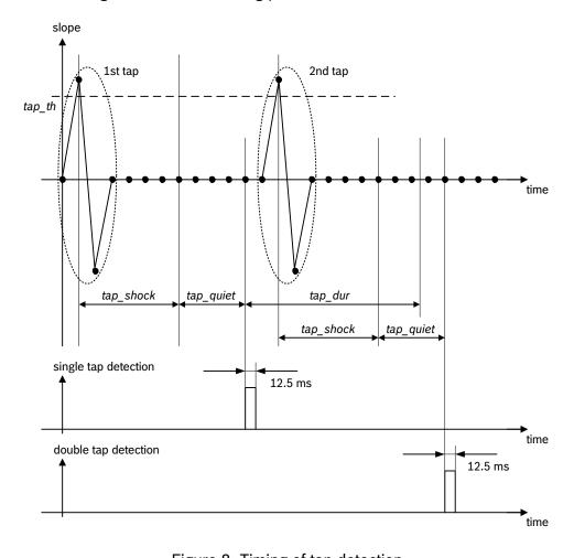
Figure 8: Timing of tap detection
