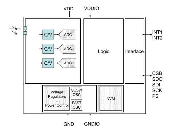
Figure 1: Block diagram of BMA253
