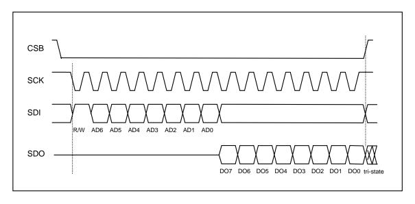
Figure 15: 4-wire basic SPI read sequence (mode '11')
