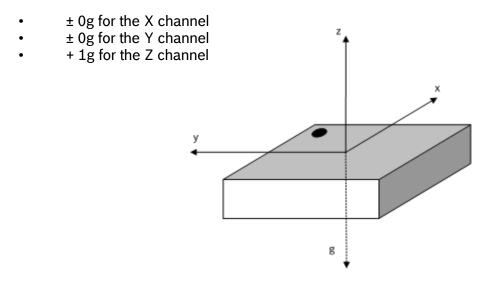
Figure 28: Orientation of sensing axis
