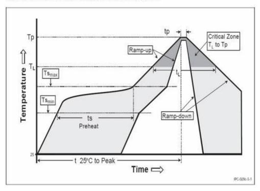
Figure 30: Soldering profile
