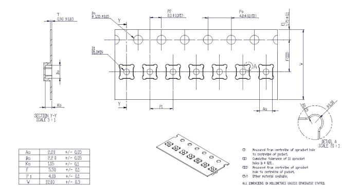
Figure 31: Tape and reel dimensions in mm
