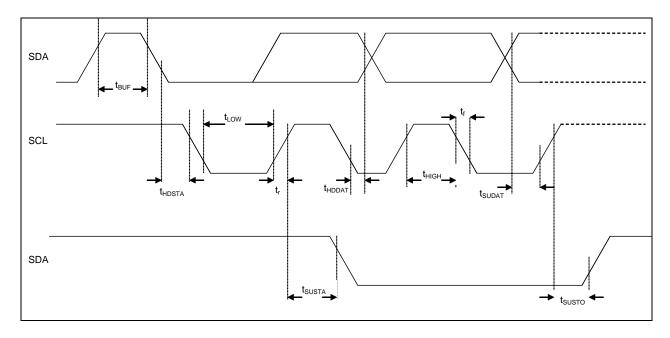
Figure 18: I2C timing diagram
