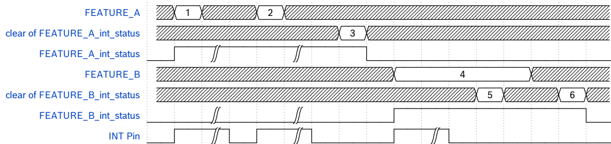
Figure 18: Interrupt output in pulses mode
