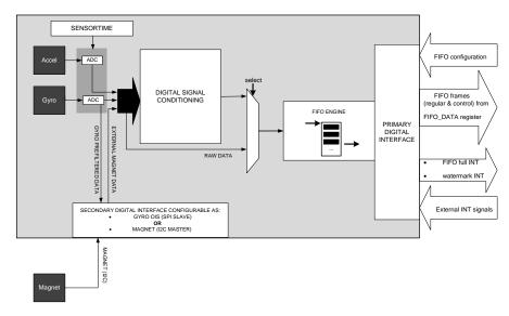
Figure 3: Block diagram of FIFO data path
