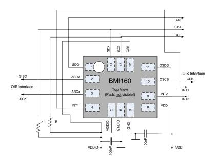
Figure 40: Using I<sup>2</sup>C and 3-wire SPI as OIS interface
