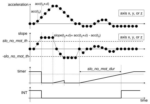
Figure 17: Signal timings no motion interrupt
