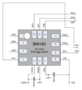
Figure 34: Only SPI 3-wire as primary interface
