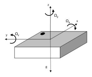
Figure 42: definition of sensing axes orientation
