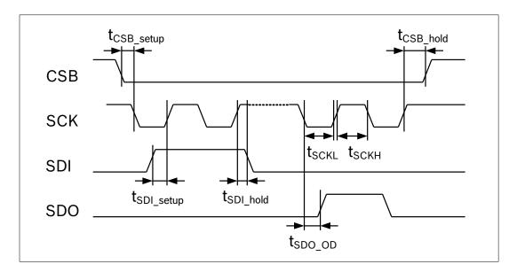
Figure 22: SPI timing diagram
