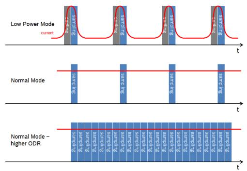
Figure 2: low power and normal mode operation
