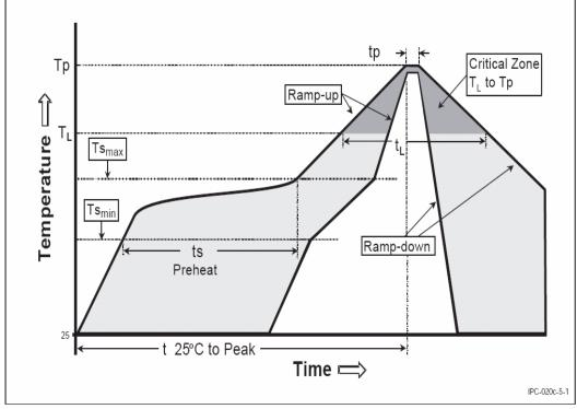
Figure 45: Soldering profile
