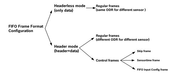
Figure 4: FIFO frame configurations
