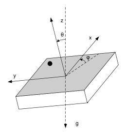
Figure 8: definition of coordinate system with respect to pin 1 marker
