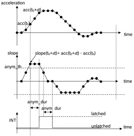
Figure 5: Any-motion (slope) interrupt detection
