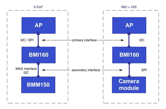
Figure 21: Examples for secondary interface usage
