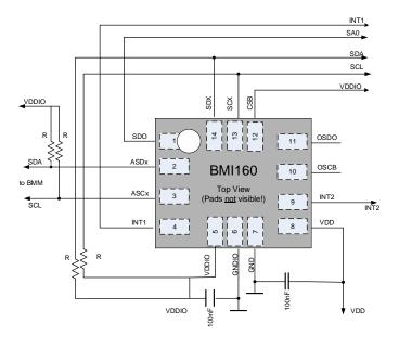
Figure 38: Using I<sup>2</sup>C and the magnetometer interface
