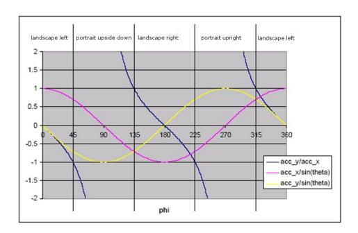
Figure 9: Angle-to-Orientation Mapping
