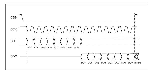
Figure 24: 4-wire basic SPI read sequence (mode '11')
