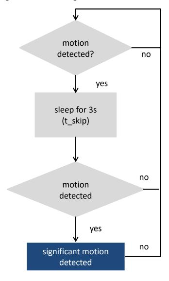
Figure 6: Block diagram of significant motion interrupt algorithm
