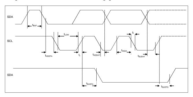
Figure 27: I2C timing diagram
