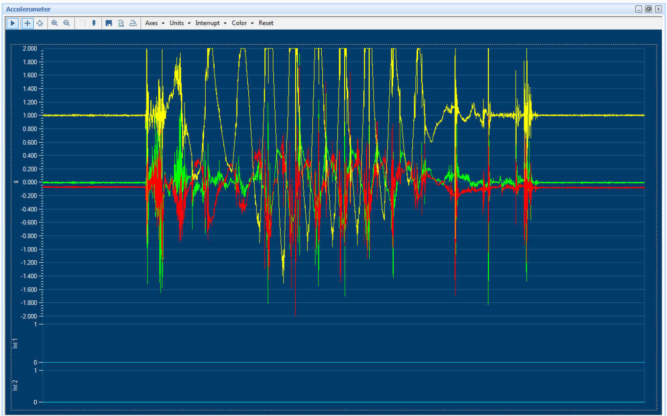
Figure 5 : Accelerometer data plotter
