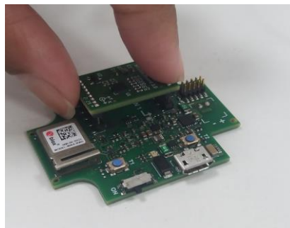
Figure 2 : Insert sensor for APP3.0
