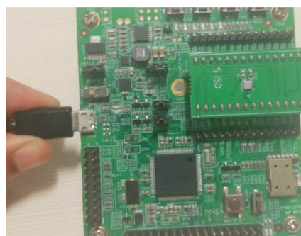
Figure 3 : Connect board and PC for APP2.0
