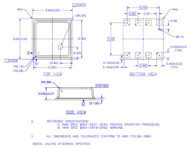
Figure 1: BME6xy package dimensions (in millimeter) for top, bottom and side view
