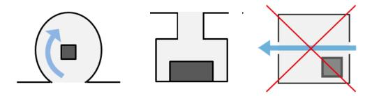
Figure 3: Cavity designs with: (left) defined air flow, (middle) small cavity, (right) large cavity volume and no direct air flow
