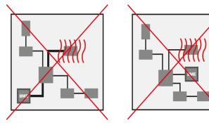
Figure 4: BME6xy placement on a PCB (red: heat radiation)
