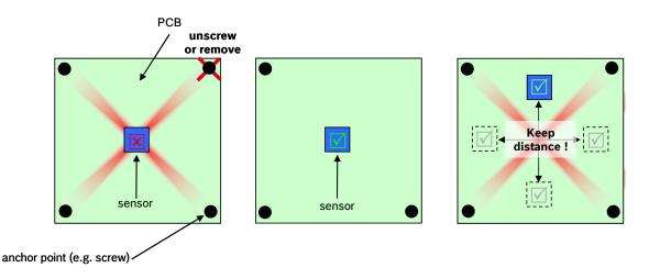
Figure 6: Methods to minimize mechanical stress on the sensor: (left) sensor is wrongly placed at a high mechanicallystressed location, (middle) redundant screw is removed to minimize stress, (right) sensor is properly placed at a reasonable distance from high mechanically-stressed areas
