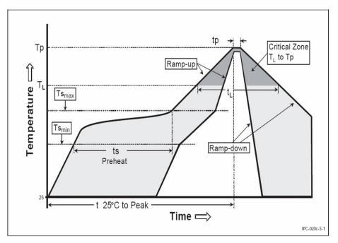
Figure 2: Soldering profile
