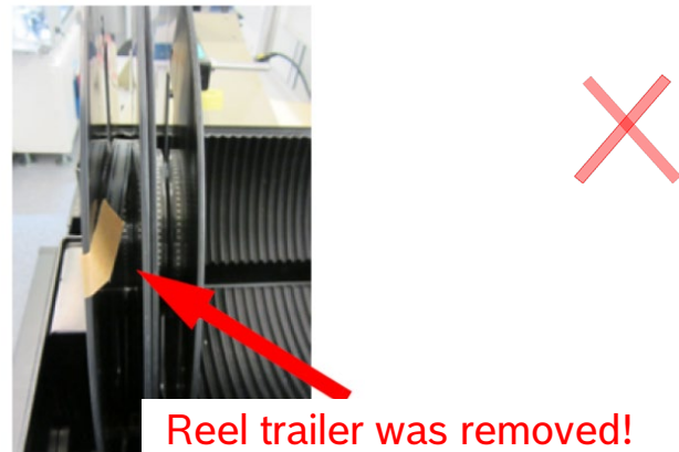
Figure 18: Reel trailers must not be removed
