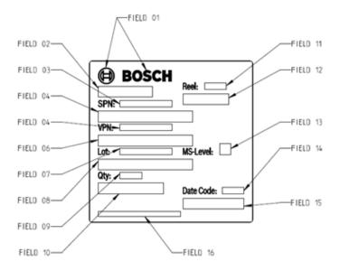
The dimension of the bar code label is approximately 72mm x 73mm (h x w).
