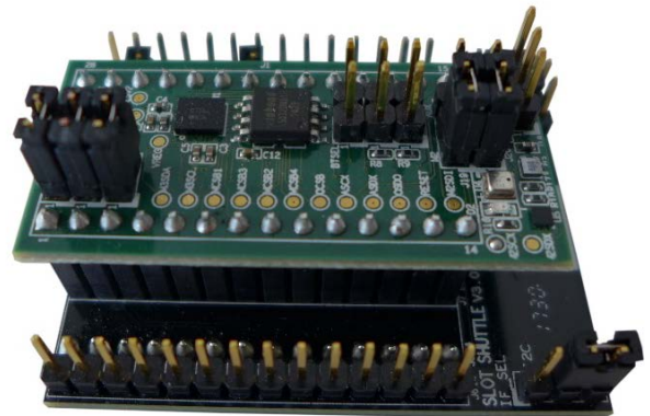
BHI260AB shuttle board mounted on level-shifter board (product photo may differ from real product appearance).
