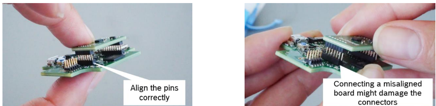
Figure 8: Aligning the pins of the Shuttle Board 3.0 board
